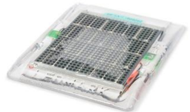
iRoad-Demo: Live Traffic Monitoring using a Road Marking Unit
